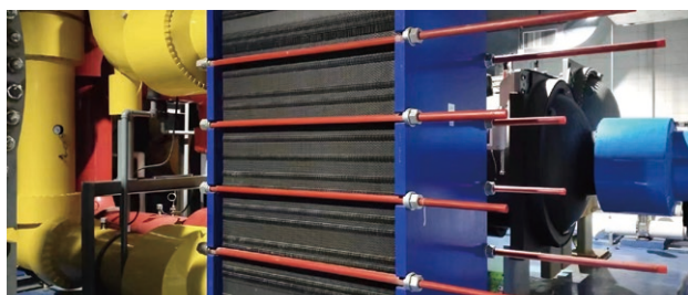
© Temperature-based control of plate heat exchanger
